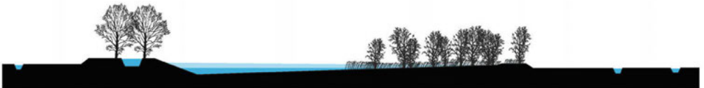
13 Extension of the carrying capacity of polder outlets: the ‘tussenboezem’, H+N+S Landscape Architects
